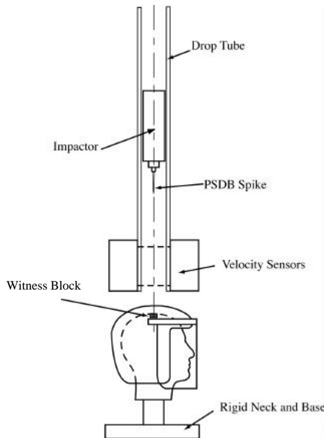
**FIGURE 8** Penetration Test
