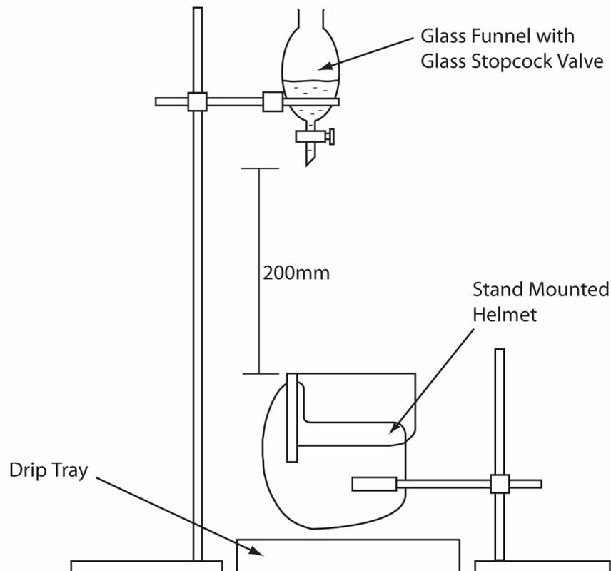
**FIGURE 16** Visor Solvent Test
