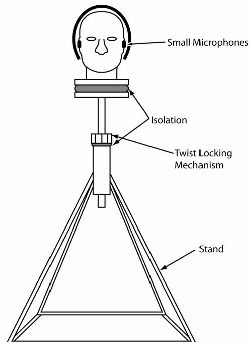
**FIGURE 5** Test Mount for Acoustic Test
