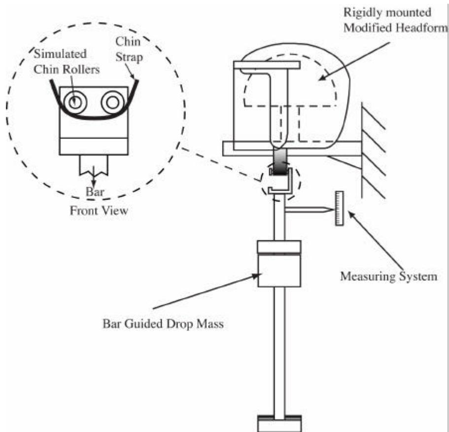
**FIGURE 7** Retention Strength Test
