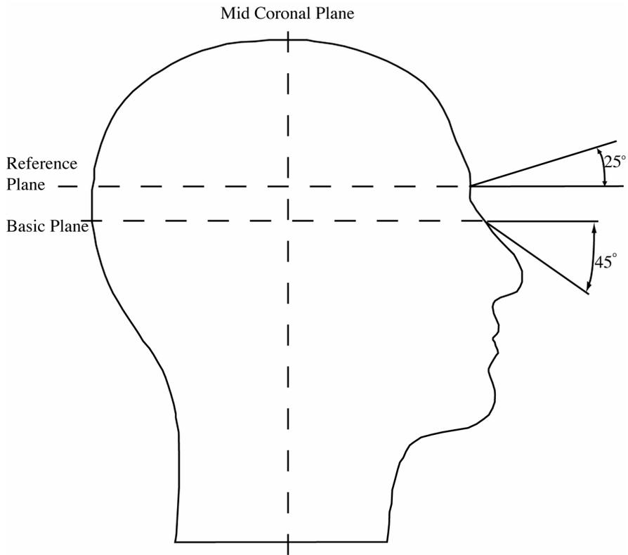
**FIGURE 3** *Peripheral Vision - Forwards*
