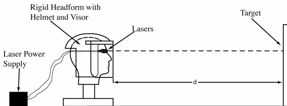
**FIGURE 11** Example Orientation of Headform and Target
