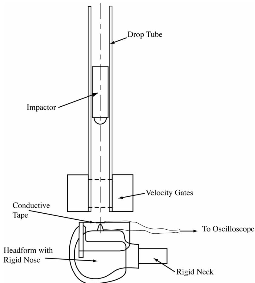
**FIGURE 14** *Visor Impact Test*
