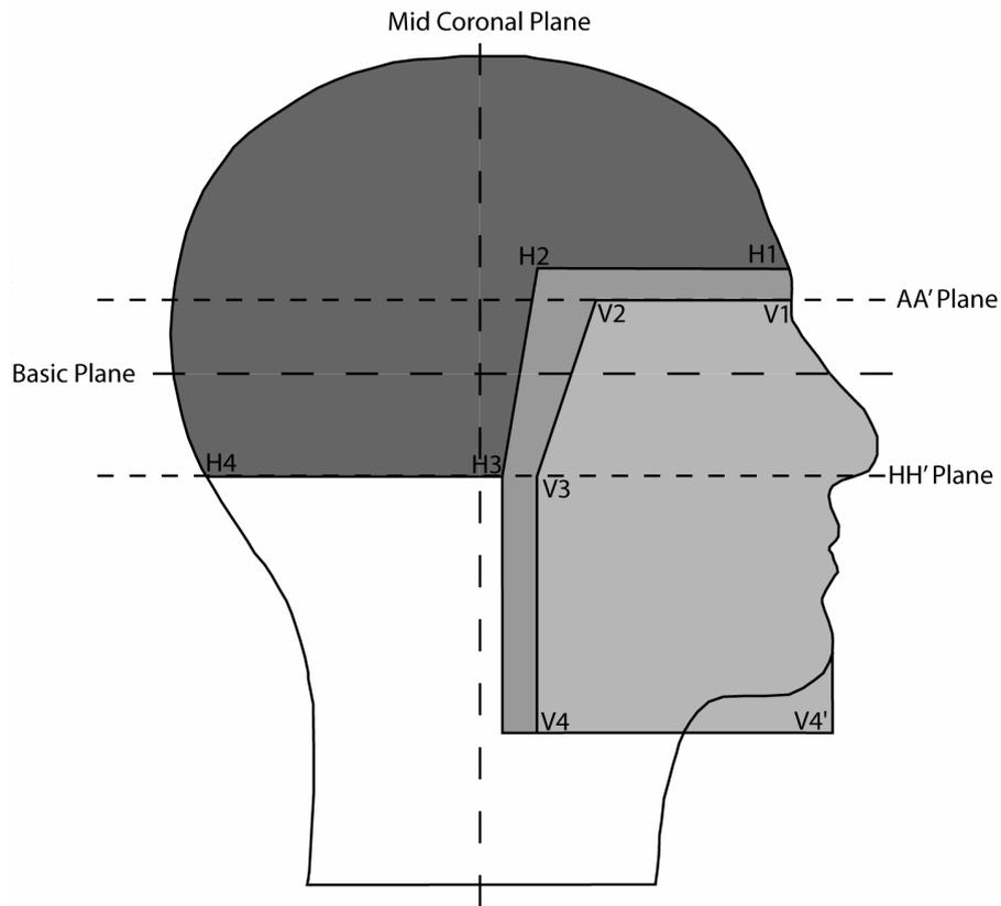
**FIGURE 2 Coverage of Helmet Body and Visor**
