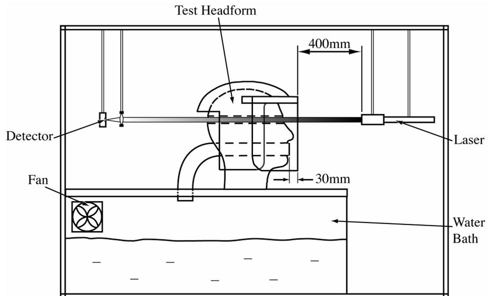
**FIGURE 13** Visor Mist Test
