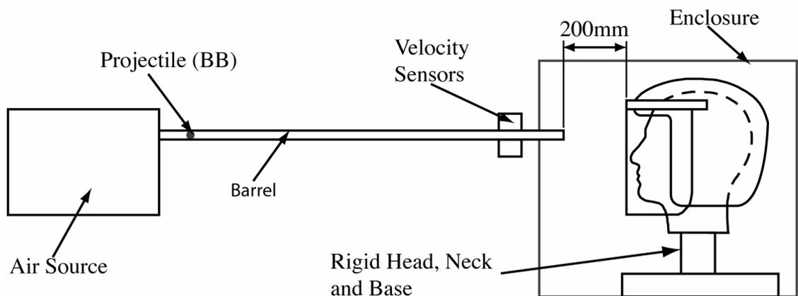
**FIGURE 15** Visor Pellet Test
