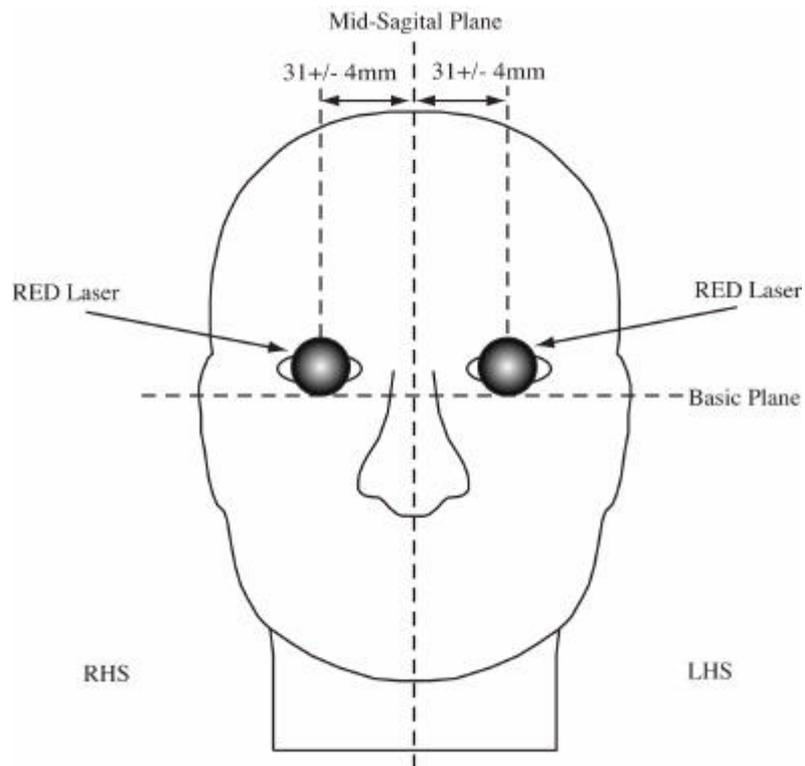
**FIGURE 10** Example Headform with Laser
