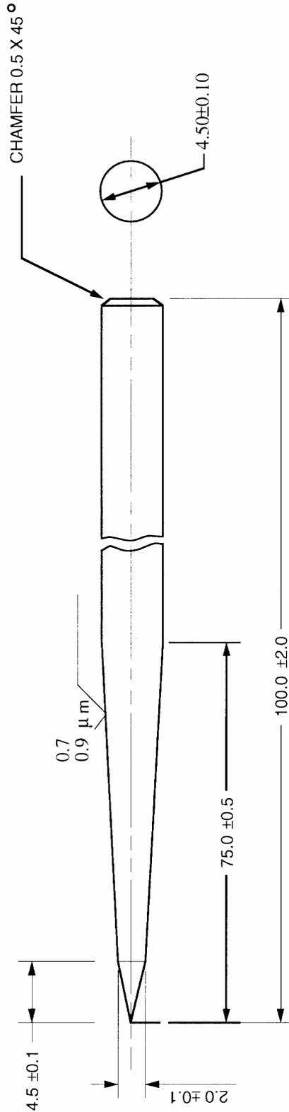
NOTE: 0.1mm MAXIMUM TIP RADIUS AFTER GRINDING
