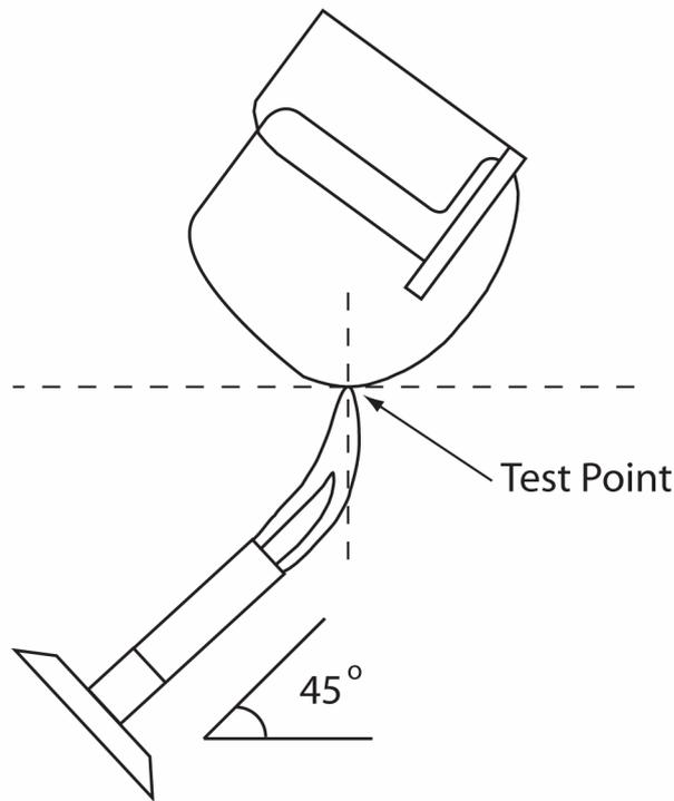
**FIGURE 6** Flame Test
